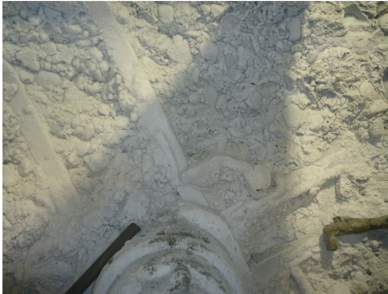
Figure 11. Frozen Interior of Cutter Head
