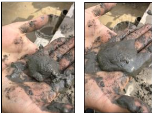
Figure 3. Silty dilatant material behavior Class C soil a) before shaking b) after shaking
