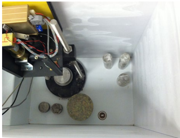
Fig. 3b. Compression test load frame in freezer
