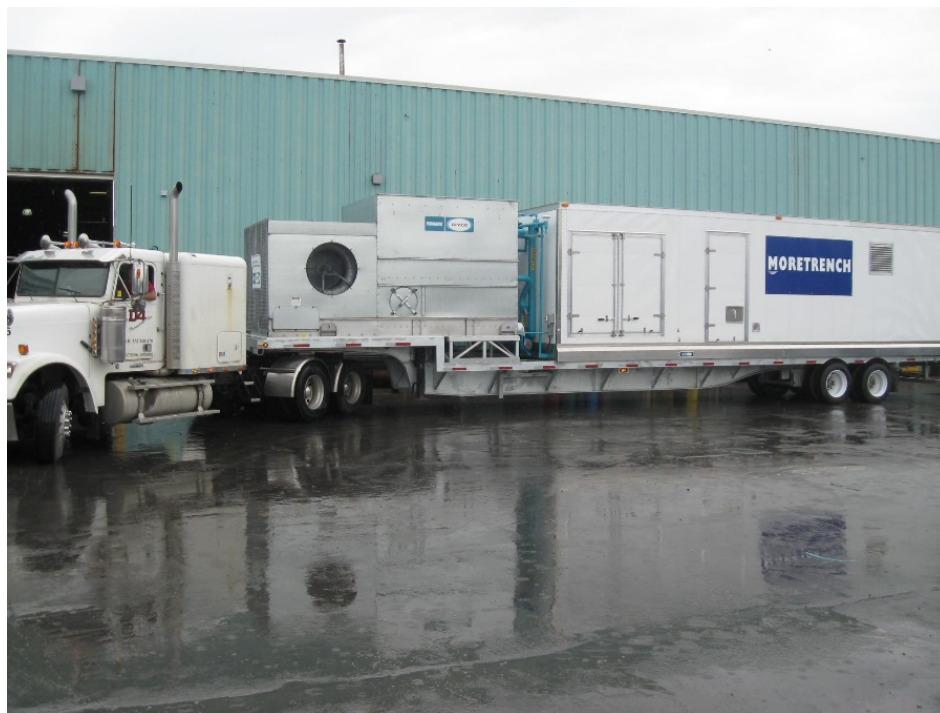
Fig. 7a. 310 kw at -30^{\circ}\text{C} refrigeration plant
